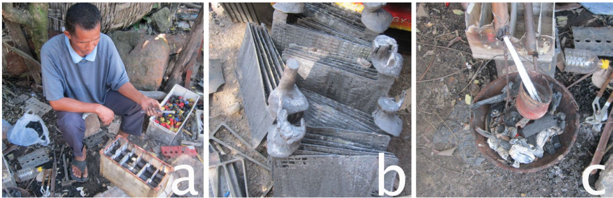
Figure 6. Lead harvesting from batteries for repurposing: a) an artisan works to remove lead-antimony plates and melt them into small pieces for resale; b) close-up view of lead-antimony plates; c) stick of Pb heated over a charcoal stove.
