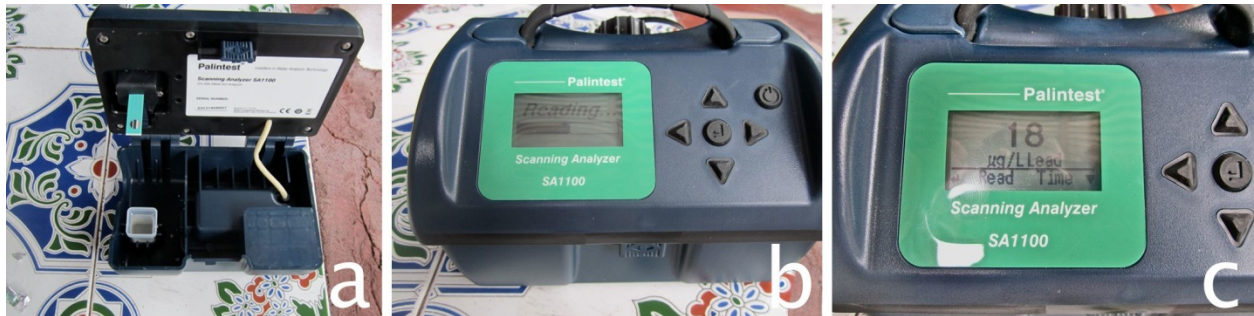
Figure 15. ASV process: a) the ASV unit with electrode in place and sample prepared; b) sample processing; c) corresponding measurement of dissolved Pb concentration.
