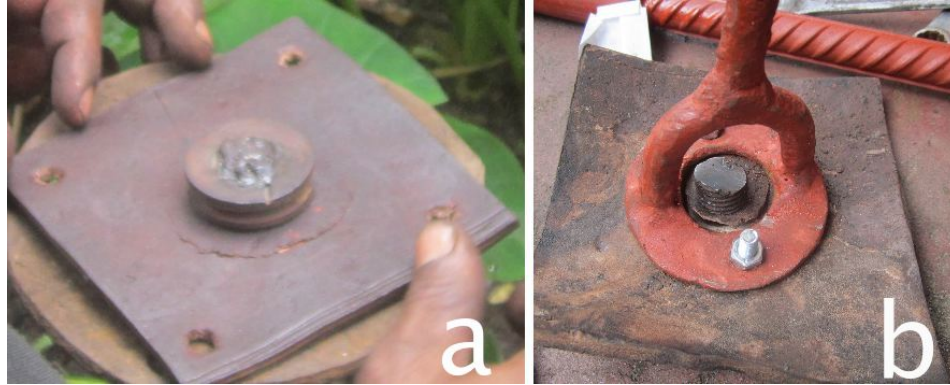
Figure 14. Alternative Fe scrap materials used in valve fabrication: a) lower (foot) valve; b) upper (piston) valve.
